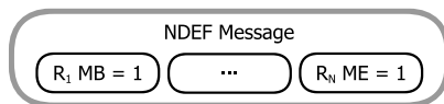
Fig. 2. Multiple records form an NDEF message. The flags MB and ME are set for the first and the last record respectively.
