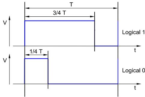
**Figure 2.** Pulse width modulation bit coding is used for master-to-slave (S1) communication [2].
