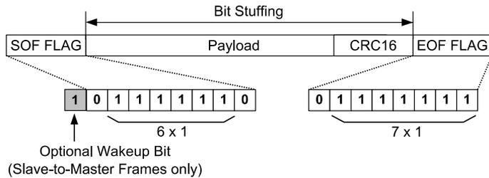
**Figure 3.** Frame structure used for data exchange on the MAC layer between master and slave [2].
