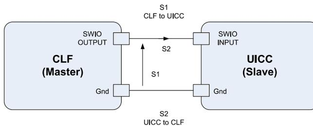
**Figure 1.** Single Wire Protocol: Data is transferred through a single wire (with a reference to ground), where S1 is the master-to-slave signal in the voltage domain and S2 is the slave-to-master signal in the current domain [2].
