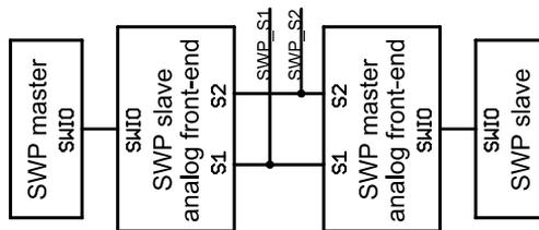
**Figure 6.** The packet sniffing circuit is composed of a master's and a slave's analog front-end.
