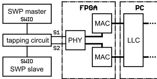
**Figure 4.** The SWP packet sniffing system consists of a tapping circuit, an FPGA with the physical transmission layer and the medium access control layer, and PC software for decoding higher layers.
