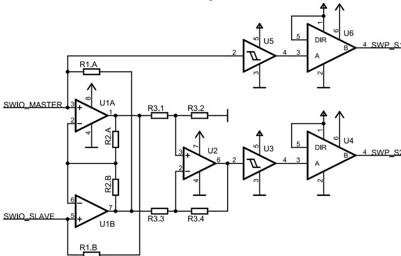
**Figure 5.** The measuring probe is composed of an ampere meter with a low voltage drop [5], [6] and Schmitt triggers to form the analog voltage signals into digital signals. Bus transceivers are used to shift the voltage levels of the digital signals to those of the FPGA. ( $R_{1,A} = R_{1,B} = R_1$ ,  $R_{2,A} = R_{2,B} = R_2$ ,  $R_{3,1} = R_{3,2} = R_{3,3} = R_{3,4} = R_3$ )
